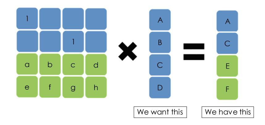
Left multiply both sides by the inverse encoding matrix
