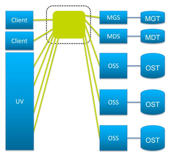
Multi-Rail LNet allows for the LNet network configuration to match the fabric.
