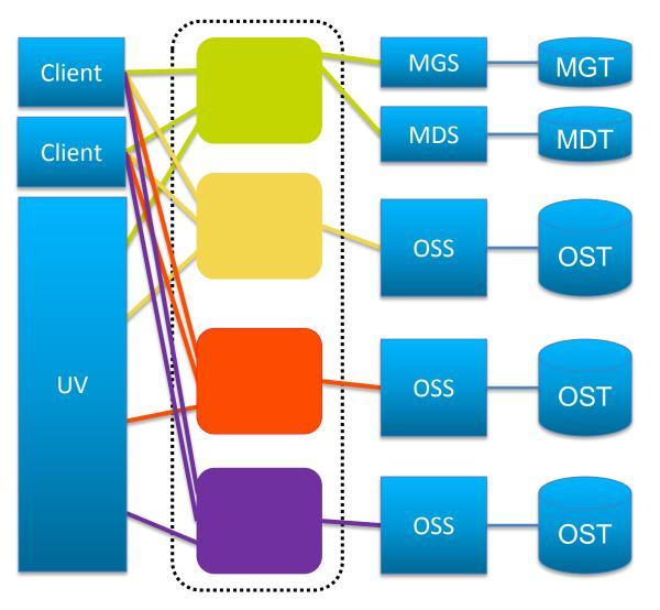
Additional interfaces have been added to the UV to increase its bandwidth.
