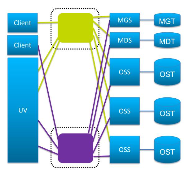
In this example there are two fabrics, each with an LNet network on top.
