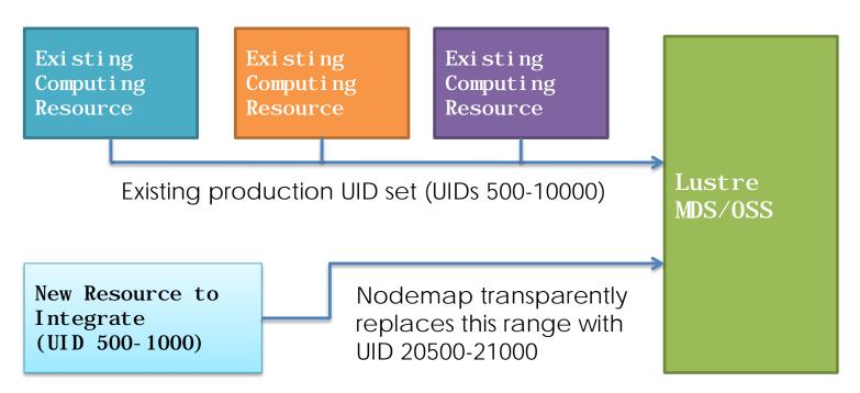
A mature Lustre system may have UID and GID sets that conflict with another system being integrated. Nodemap enables that system to be seamlessly mounted to the existing Lustre installation.
