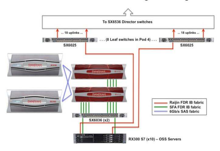
Fully redundant SAS enclosures, FDR IB between storage and OSSes and uplinks to Raijin
